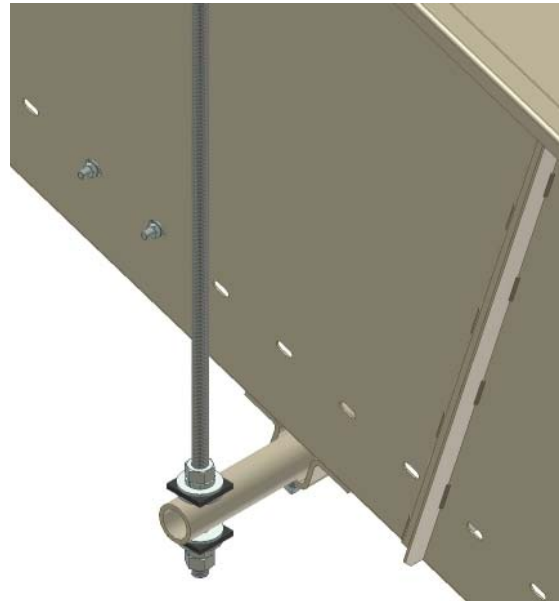
Overhead Decline Support with Pipe Sill
